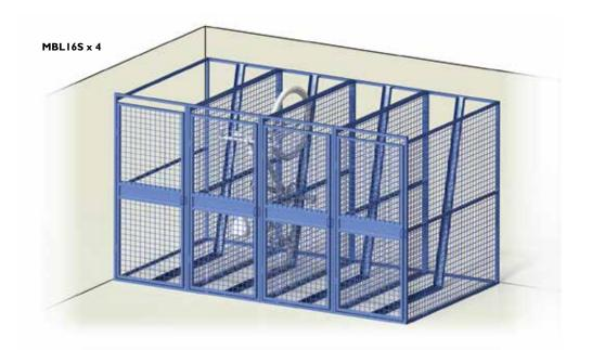
$\begin{tabular}{ll} \textbf{Material Specifications (General)} \\ \textbf{MBL16S} & 25 \times 25 \times 1.6 \text{mm SHS} / 50 \times 50 \times 4 \text{mm steel mesh} / \text{Galvanised} / \text{Powder coated in a range of colours} \\ \textbf{Wheel rail, vandal-proof lock, 3-way locking, optional back \& roof panels} \\ \end{tabular}$
