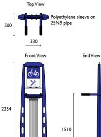
Should be installed at least 500mm from any wall
